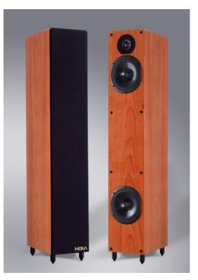
$6\frac{1}{2}$  inch bass drivers and one high resolution silk soft dome tweeter in a vertical array. Each bass driver is housed in a separate chamber and is individually ported. This technique, while costly, eliminates driver interference and provides increased clarity. The upper driver is ported to the rear, while the lower driver is loaded by a downward firing port. The chambers are tuned to different frequencies to provide the smoothest and most extended inroom bass response.
